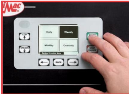
tasks for the week are displayed automatically each Monday upon start-up. A quick review of management reports can identify problems before operators are aware of them. For example, an engineer can identify the current water temperature or the actual cylinder speed with a simple touch of a keypad.
