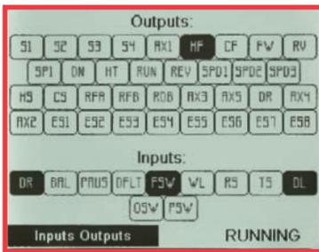
When service is required, troubleshooting is streamlined through the special diagnostic screen identifying specific functions. A banner visible during start-up of the washer displays your service company's contact information.
