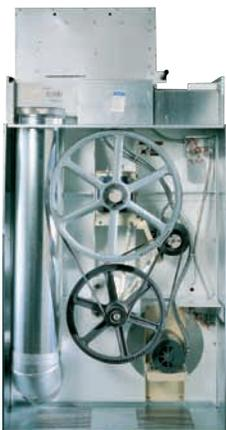
UniMac tumblers feature an all-belt drive system with easy adjusting tension idler, cast iron pulleys and permanently sealed ball bearings for quiet, low maintenance operation. As an added benefit, UniMac incorporates a solid-state electronic timer that is designed to automatically reverse the tumble action if you choose. This feature can be easily selected and aids in preventing the tangling of linens.
